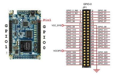
Here is the connection map between LCD and GPIO-0:
